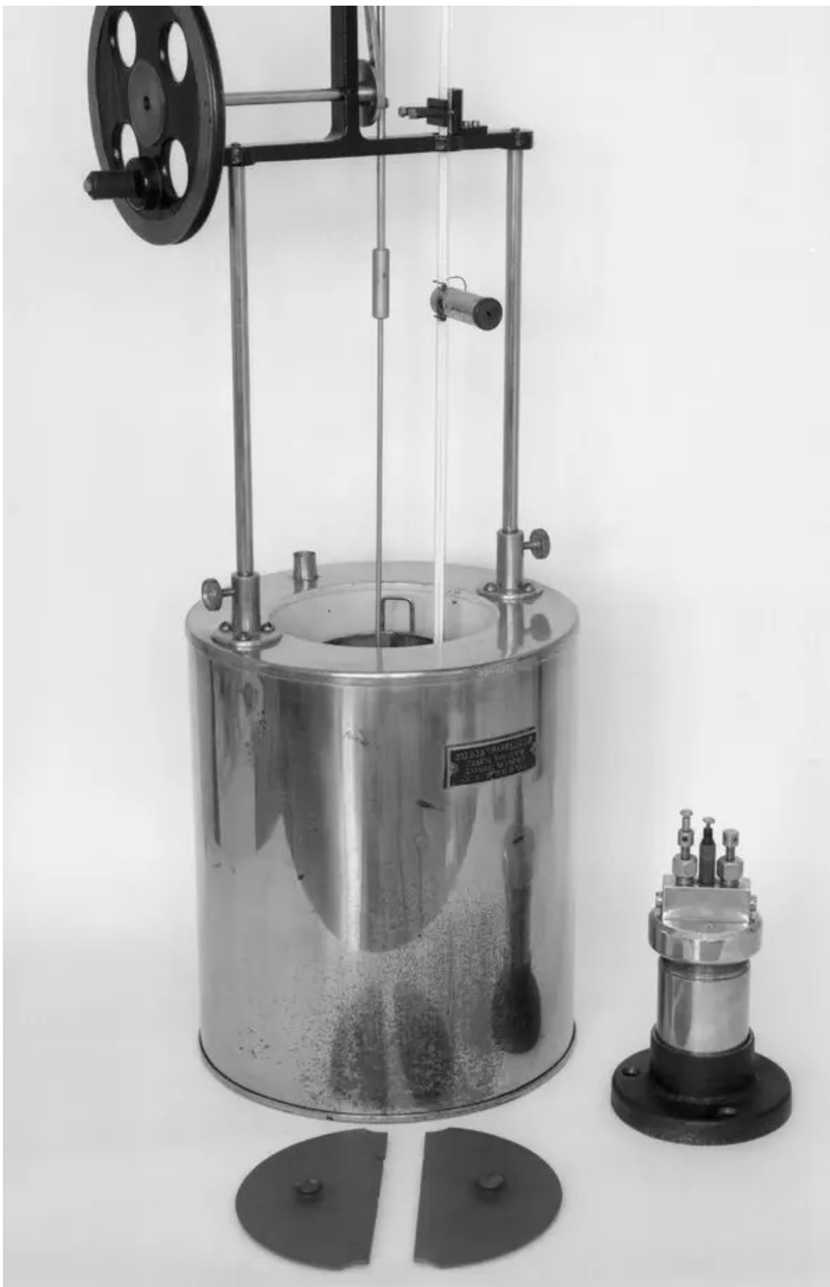
The bomb calorimeter, like this one is from the 1920s, was used to
